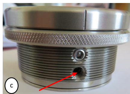
Figure 4: a) Insert with Specimen Locking Screw Hole shown; b) Slide Holder over Insert; c) Align Specimen Locking Screw holes in Insert and Holder
