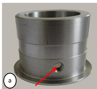
Figure 4: a) Insert with Specimen Locking Screw Hole shown; b) Slide Holder over Insert; c) Align Specimen Locking Screw holes in Insert and Holder
