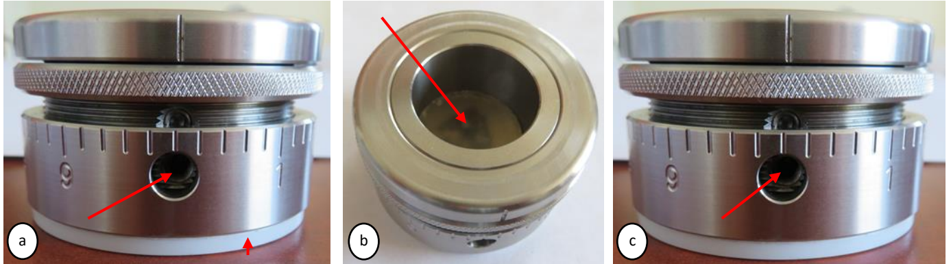
Figure 6: Installing the Specimen: a) Specimen Holder on Tabletop, Ceramic Ring Down, Specimen Locking Screw Holes Aligned; b) Specimen Inserted, Side to be Ground Facing Down; c) Specimen Secured with Specimen Locking Screw
