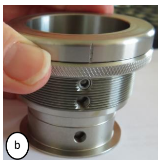
Figure 4: a) Insert with Specimen Locking Screw Hole shown; b) Slide Holder over Insert; c) Align Specimen Locking Screw holes in Insert and Holder
