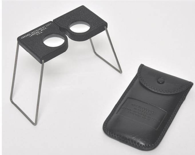
The #758 Stereo Viewer is a folding, pocket sized viewer which is ideal for three dimensional viewing of stereomicrographs. The precision ground and coated lenses give a two times magnification. A simple interpupillary adjustment calibrated in millimeters is provided. The viewer is packed in a protective carrying case.
