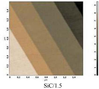
6H-SiC (0001) based calibration sample which is designed to perform easy calibrations of an AFM scanner vertical movements in several nanometers interval. The simplicity of calibration of the calibration process is provided by the nearly uniform distribution of half-monolayer high steps (either 0.75 or 1.5nm) on the sample surface demonstrating both chemical and mechanical stability. The step height corresponds to the half of the lattice constant of the 6H-SiC crystal in the (0001) direction.
