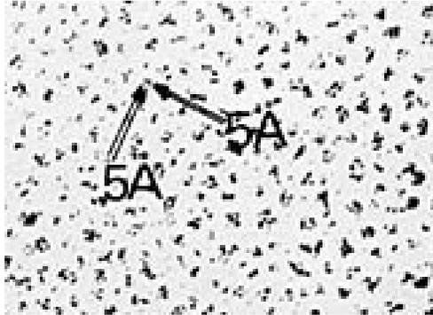
This specimen may be used to test the resolution of the electron microscope by the point separation test. The distance between the centers of two small particles, which can just be distinguished as separate, can be taken as a measure of the resolution.
