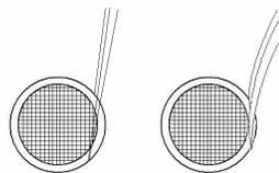
Slot grids should best be gripped by curved tweezers
