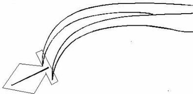
Mesh grids can be gripped by straight or curved tweezers
