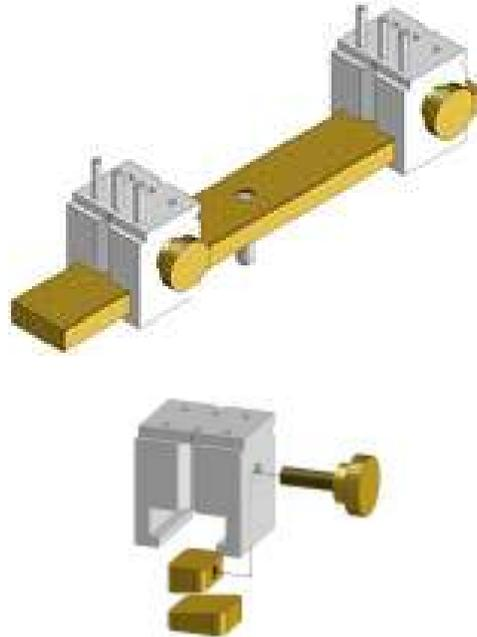
**Release jaws by loosening the thumb screw and pressing it in to unlock the wedge holding it to the bar.**
