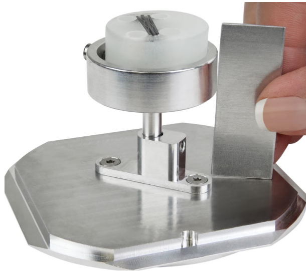
Figure 3: 50mm height gauge being used to check the sample height.
