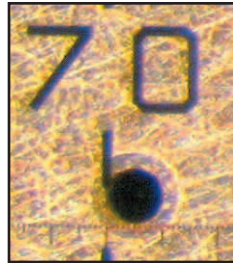
100µm aperture... the scale is down this time, placed on top of an aperture and photographed. The aperture diameter is 100µm.
