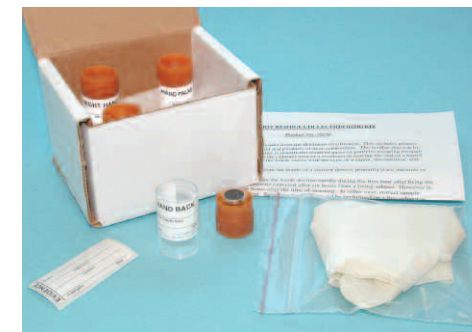
4-Disc GSR Field Kit suitable for sampling palm and back separately on both hands. Prod. No. 16256-4
