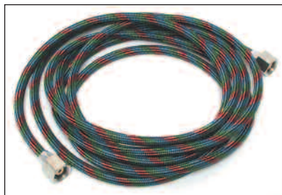
803 Flex Air Hose, extremely flexible, 10' long, Nylon-covered braided air hose with 1/4" NPT female ends.
