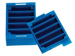
The CellSafe™ is designed to contain small tissue fragments and biopsies during tissue processing. The CellSafe™ 5 was developed for the simultaneous preparation of core needle biopsies. Each well is numbered for identification. The blue cassette aids with contrast and visualization of light colored biopy tissues.
