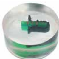
Example: Circuit board encapsulated using the PELCO® Epoxy Mount Kit.
