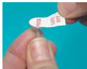
adhesive being applied to a specimen mount using Lift-N-Press Tabs
