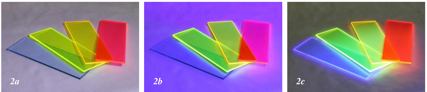
Figure 2: Technovit® Blue LED Flashlight 2.0 Flashlight Settings (2a) One Click: White Light; (2b) Two Clicks: Blue Light; (2c) Three Clicks: Purple Light
