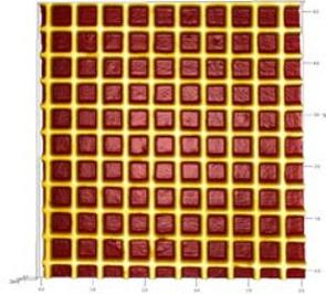
The height of the bars of the grid pattern is approximately 100nm. To calibrate instrument magnification, use the following calculation:
