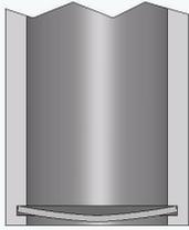
Fig. 1. The screen in each well fits into a recessed groove as shown. The screen can be removed by using a flat/blunt object like a pencil eraser to push the screen out. A new screen is put in place by inserting it into the top of the well and gently pushing down with the eraser end of a pencil or similar blunt object.
