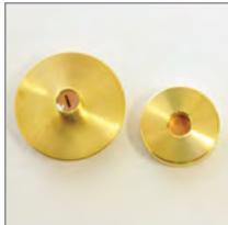
6. TEM grid shown placed into recess in grid holder top.
