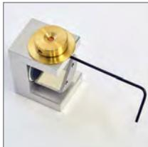
8. Replace grid holder unit into base and tighten set screw.
