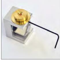
2. Loosen set screw base and remove TEM grid holder with aperture.
