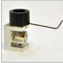
1. Loosen set screw and remove anti-scatter sleeve.
