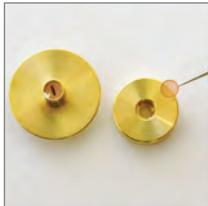
5. Place 3.05mm TEM grid into recess in grid holder top, sample side down (will be incident beam side up when installed in microscope).
