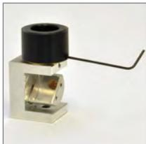
9. Replace anti-scatter sleeve onto base, over grid holder and tighten set screw.
